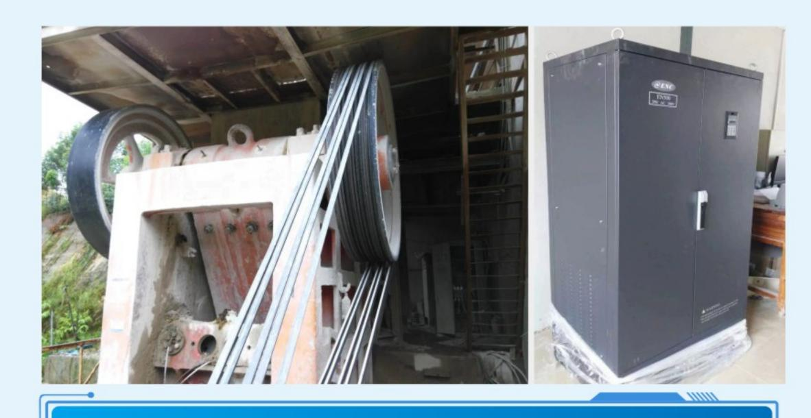
Crusher, using EN500 series inverter
