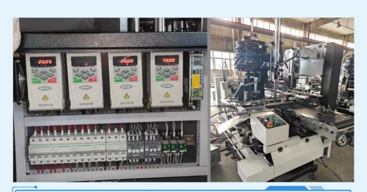
Fully automatic top and bottom paper box forming machine, using ENA100 series inverter
