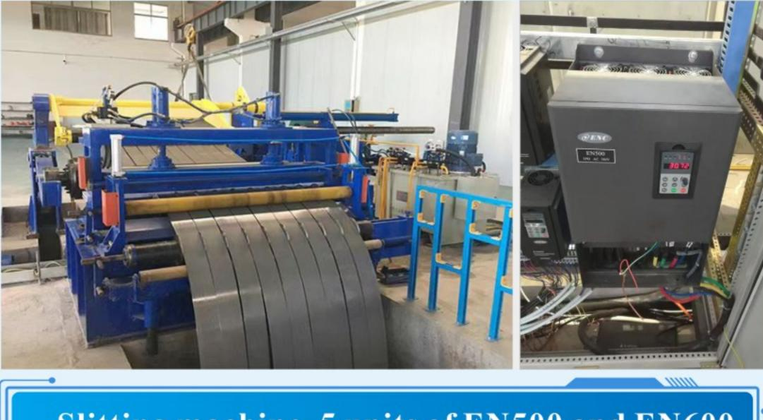
Slitting machine, 5 units of EN500 and EN600 series inverters are used on site
