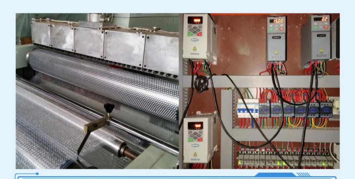
Bubble film machinery, using EN750 and ENA100 series inverters
