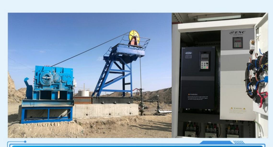
Winch-type oil pumping unit, using EN600 series inverter
